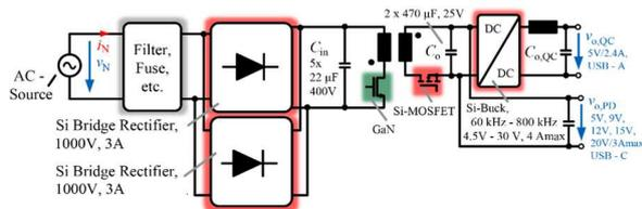
Fig. 4: Basic schematic of the GaN A power supply with PD and QC port.
