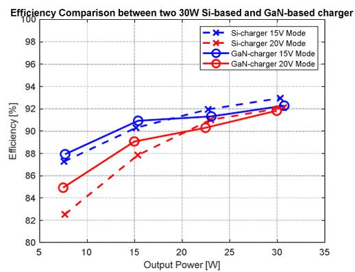
Fig. 13: Efficiency Comparison between two 30W Si-based and GaN-based chargers.
