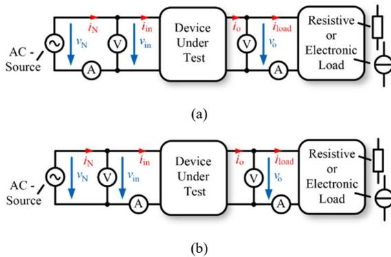
Fig. 2: (a) Measurement setup 1: voltage and current probe arrangement for a DUT (AC/DC converter) supplied from an AC-source for high power loads. (b) Measurement setup 2: Voltage and current probe arrangement for a DUT (AC/DC converter) supplied from an AC-source for low power loads.
