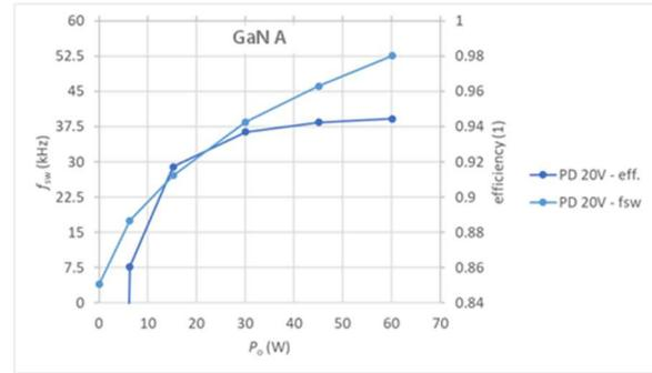
Fig. 5: GaN A port electrical efficiency and DC/DC flyback converter switching frequency of dedicated primary-side GaN transistor for different load conditions (0 W – 60 W) and a charging voltage of 20 V.
