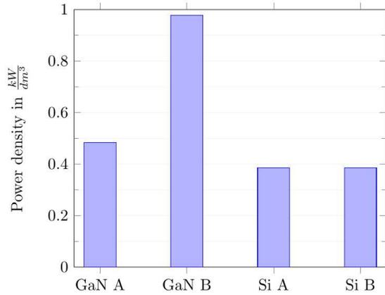
Fig. 11: Power density of the different chargers
