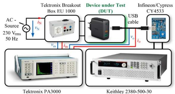
Fig. 3: Test setup including measurement devices, source, load and power analyzer.
