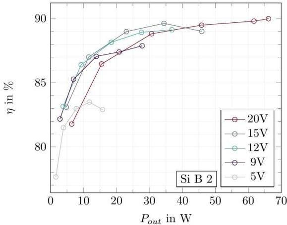
Fig. 9: Efficiency over output power curves of Si B 65W charger output, for charging voltages 5 V, 9 V, 12 V, 15 V, 20 V.
