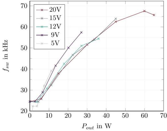
Fig. 8: DC/DC flyback converter transistor switching frequency of Si B for different load conditions (0 W – 60 W) and charging voltage levels (5 V – 20 V).
