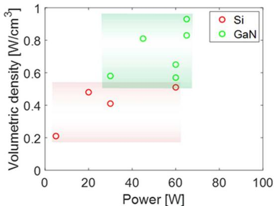
Fig. 16: Comparison of power densities of the investigated chargers.
