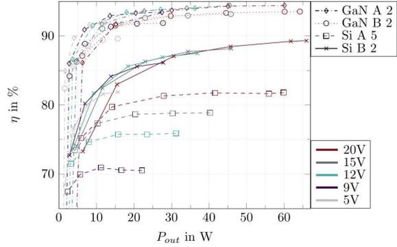
Fig. 10: Output power and efficiency of the different chargers.
