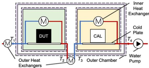
Fig. 12: Schematic view of the calorimeter.
