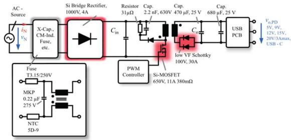
Fig. 7: Basic schematic of the Si B power supply.
