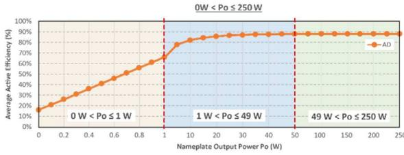
Fig. 1: Minimum limit of average active efficiency for external power supplies for a nameplate output power in the range of  $0\text{ W} < P_o \leq 250\text{ W}$  AC-DC external power supplies (AD).
