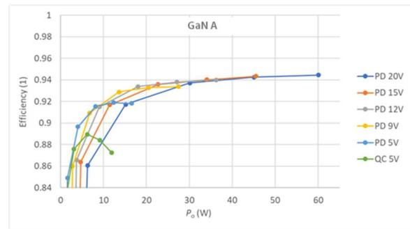
Fig. 6: Efficiency over output power curves of GaN A charger output, for charging voltages 5 V, 9 V, 12 V, 15 V, 20 V.
