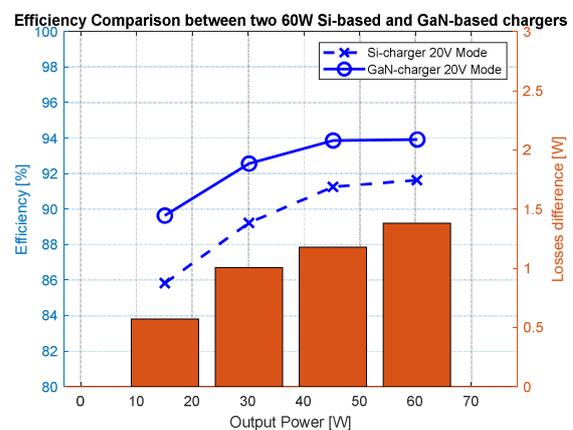
Fig. 14: Efficiency Comparison between two 60W Si-based and GaN-based chargers.
