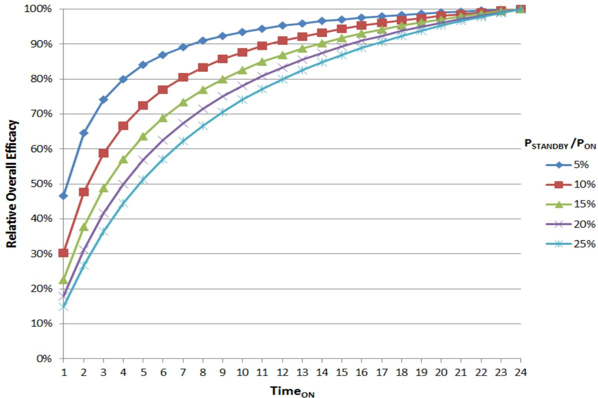
**Figure 3. Relative overall efficacy for  $P_{\text{STANDBY}}/P_{\text{ON}}$  being 5, 10, 15, 20 or 25 %**
