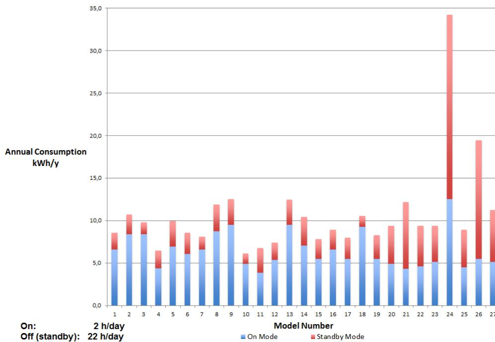
Figure 14. Annual energy consumption for 27 smart lamps models in operation 2 hours/day
