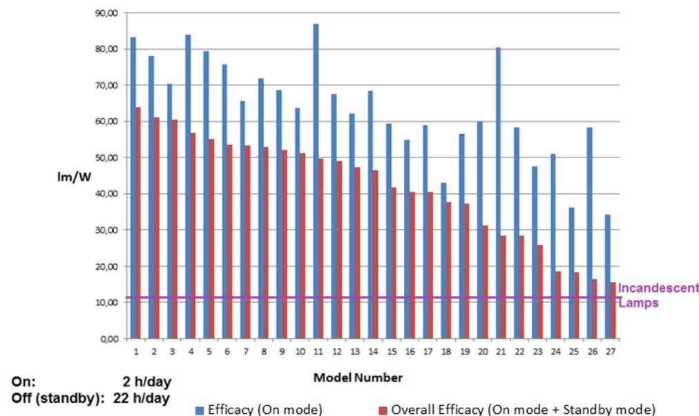
Figure 18. ON efficacy and overall efficacy for 27 smart lamps models in operation 2 hours/day
