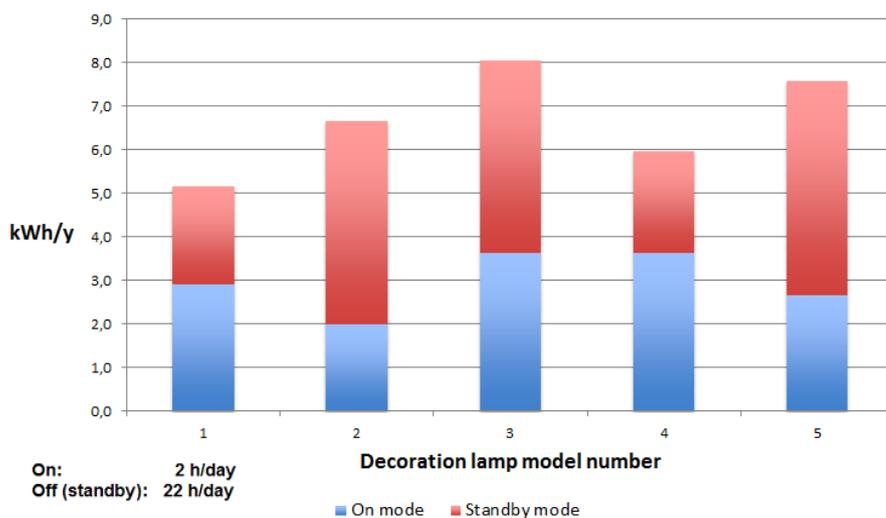
Figure 16. Annual energy consumption for 5 decoration smart lamps in operation 2 hours/day
