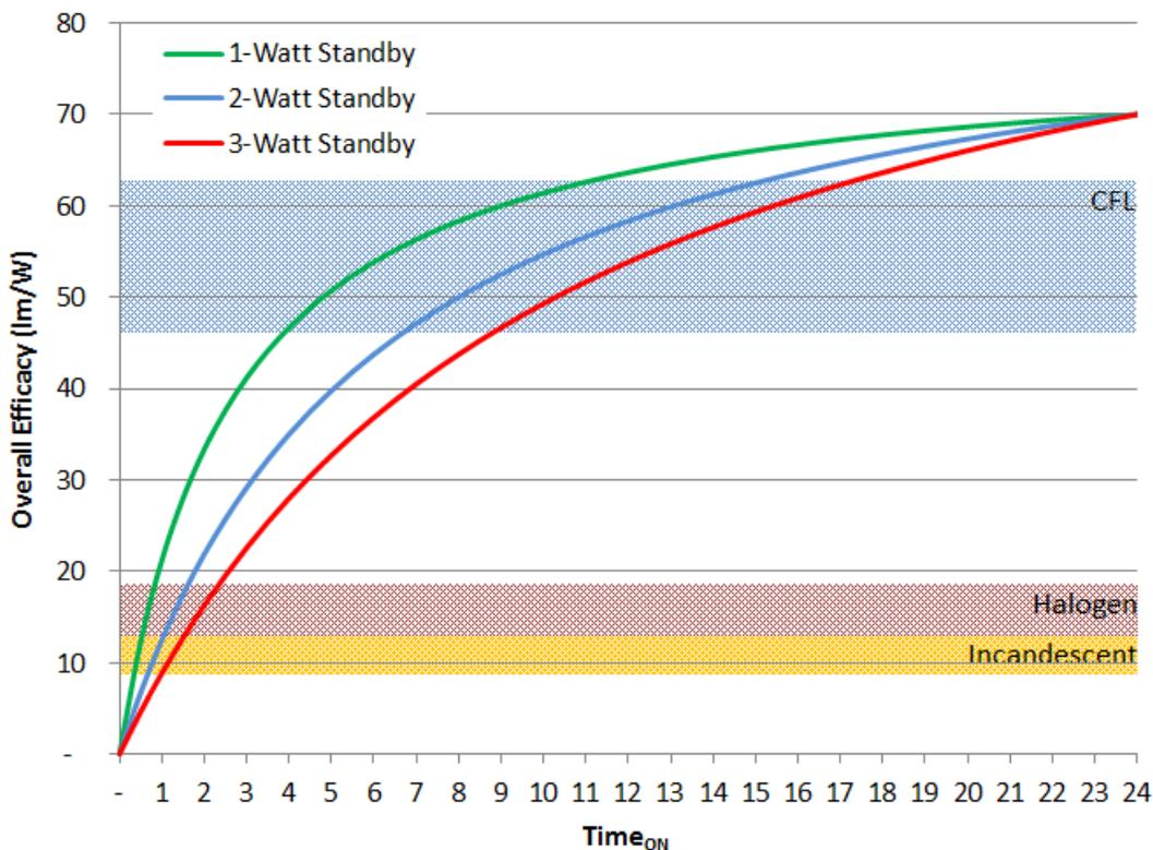
**Figure 2. Example of variation in overall efficacy of three 10 W smart lamps providing 700 lm with different standby powers (1, 2 or 3 W) for all hours of ON usage per day**
