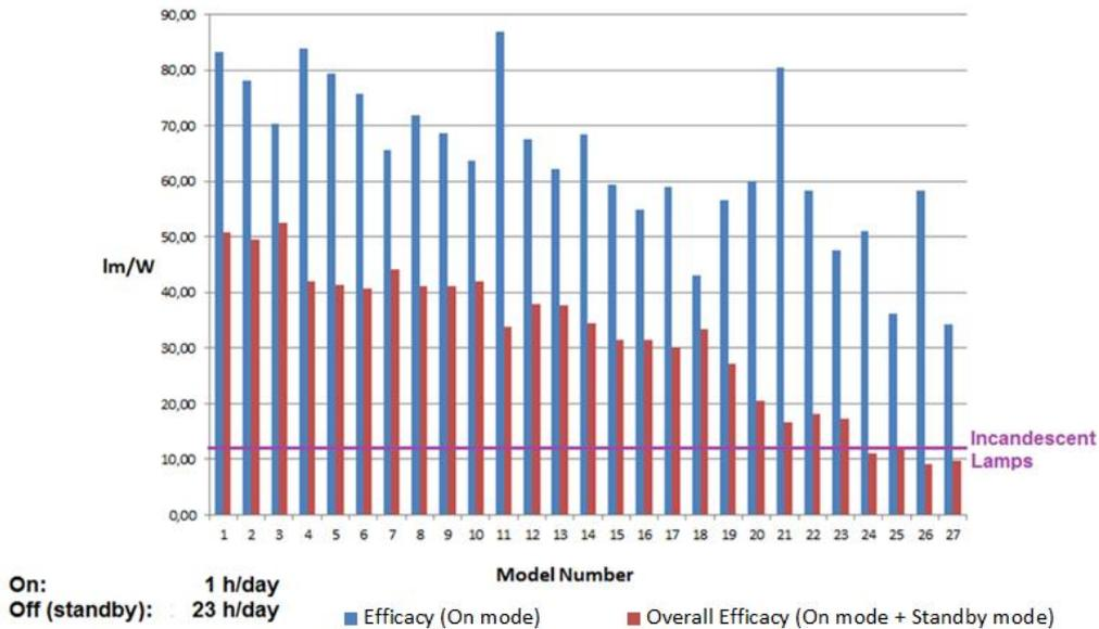
Figure 17. ON efficacy and overall efficacy for 27 smart lamps models in operation 1 hour/day
