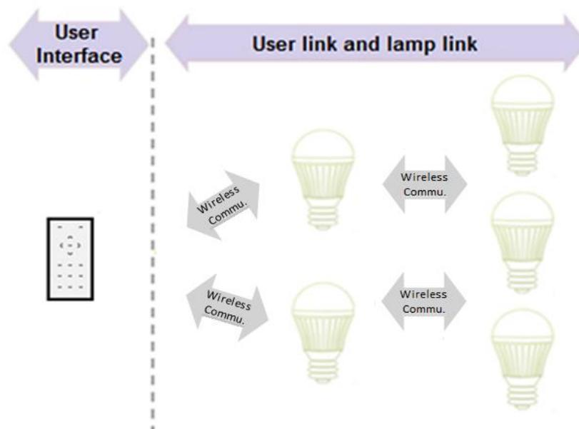
*Figure 7. Communications architecture Type D using a remote control and a proprietary protocol*
