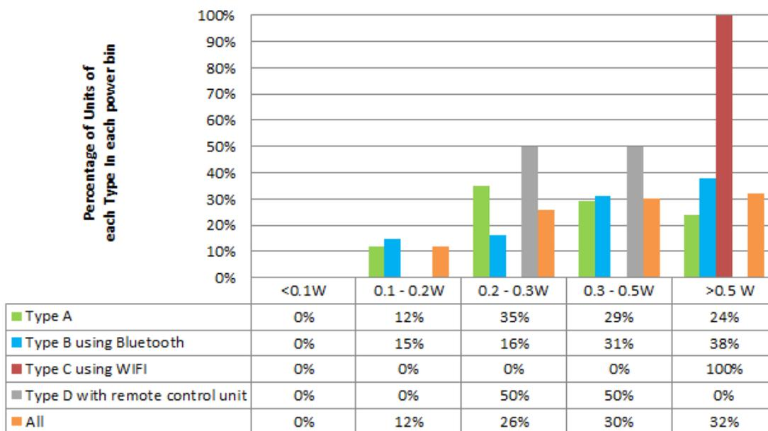
**Figure 12. Standby power consumption analysis – proportion of models in each power bin**
