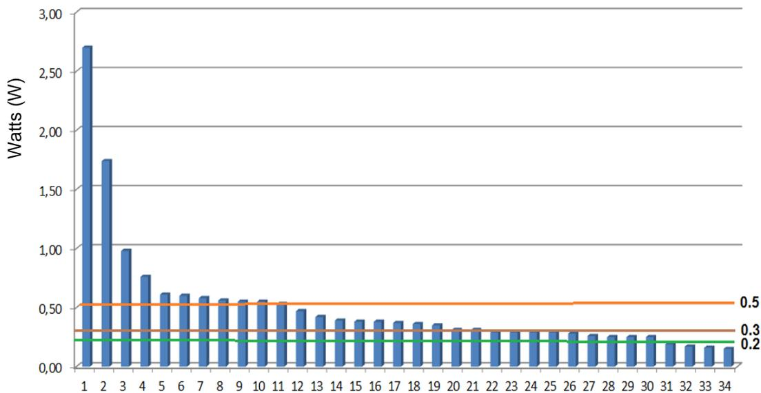
Figure 11. Standby power consumption for smart lamps
