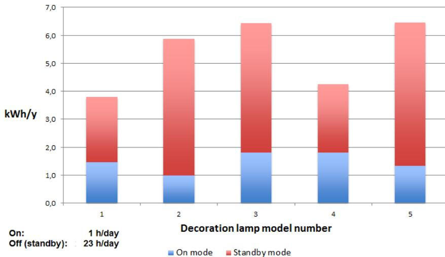
Figure 15. Annual energy consumption for 5 decoration smart lamps in operation 1 hour/day
