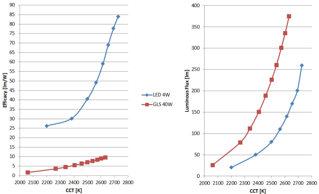
Figure 21. Comparison of DimTone LED lamp and 40 W incandescent lamp
