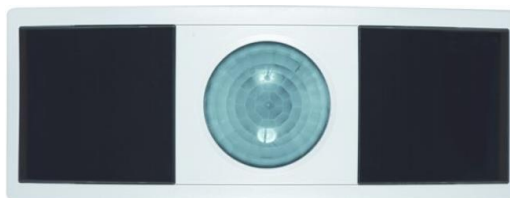
Figure 12: Self-powered wireless occupancy sensor [32].
