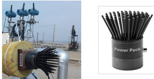
Figure 20: Self-powered outdoor temperature sensor [41]
