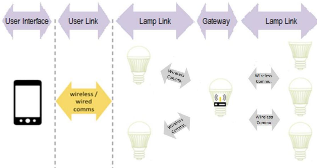
Figure 6. Communications architecture Type C using WiFi and one lamp including gateway that communicate to the other lamps using another protocol
