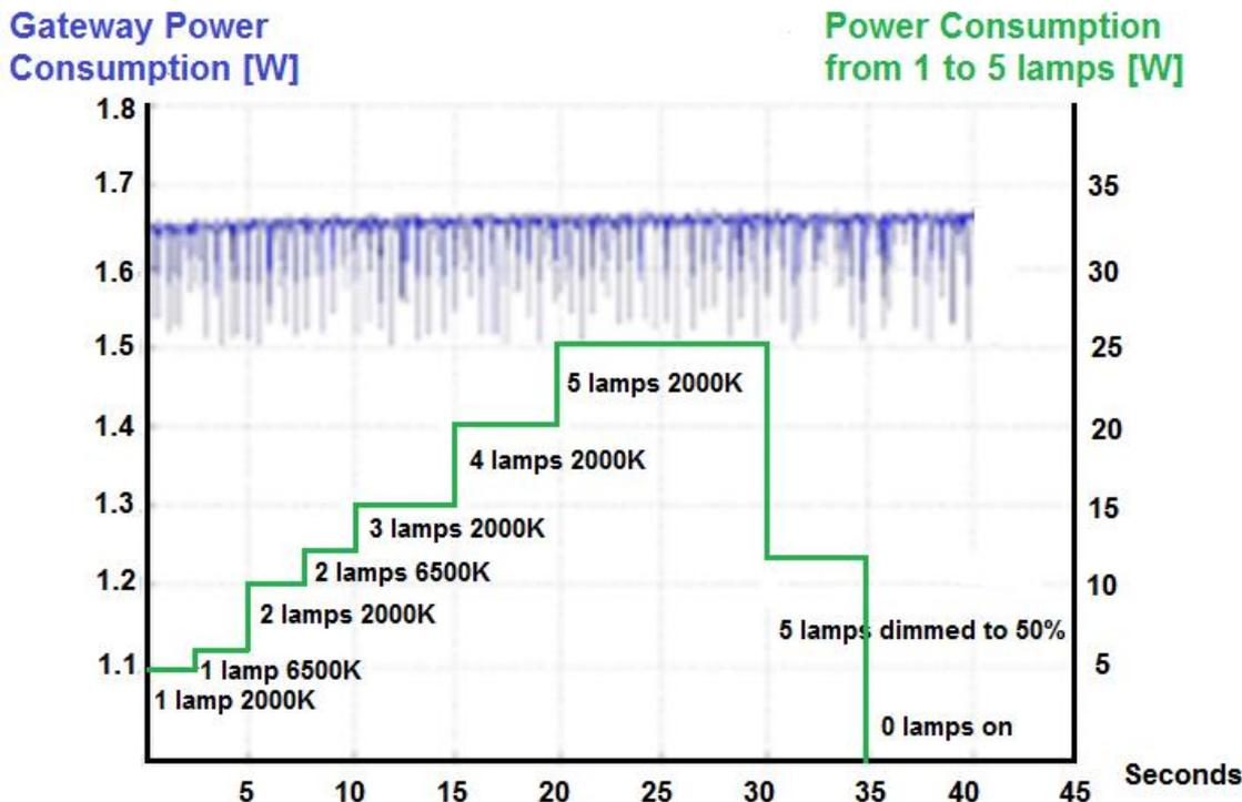
Figure 9. Nearly constant gateway consumption with a varying number of lamps in operation
