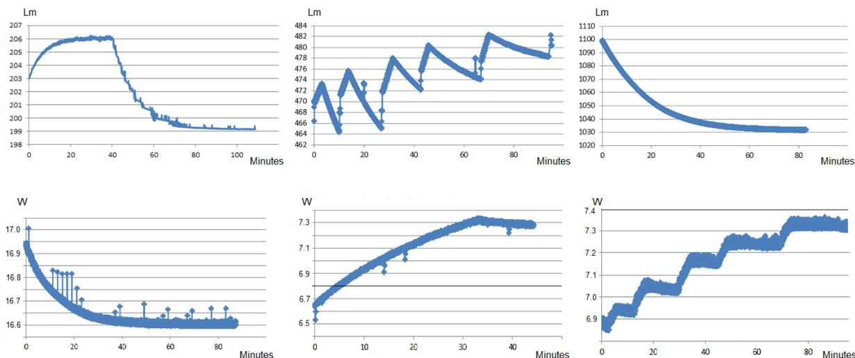
Figure 8. Examples of stabilisation measurements for luminous flux and power
