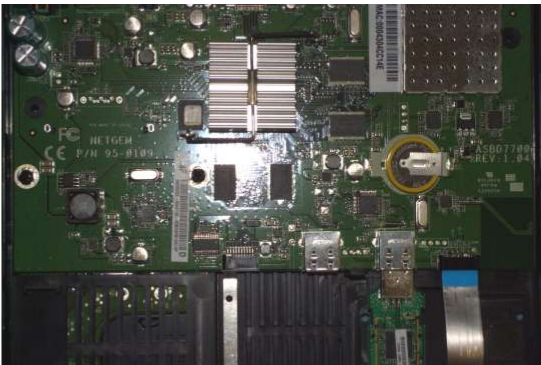
Figure 14: Circuit board for the Telstra T-Box
