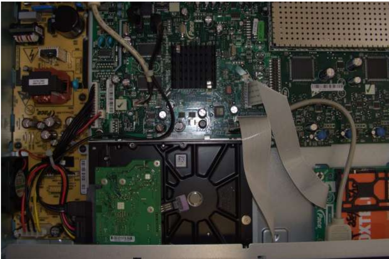
Figure 6: Photo showing the construction of the IQ2 STB.
