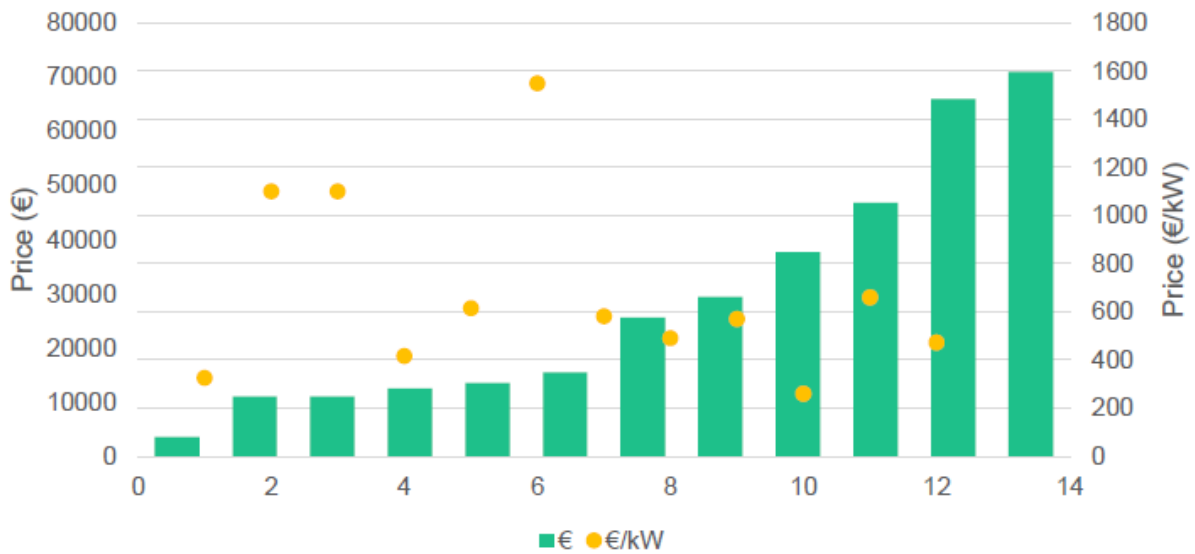
Fig. 12. Price Vs. Power for different DC recharging points [8]
