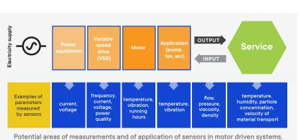
s of measurements and of application of sensors in motor driven Source: Austrian Energy Agency
