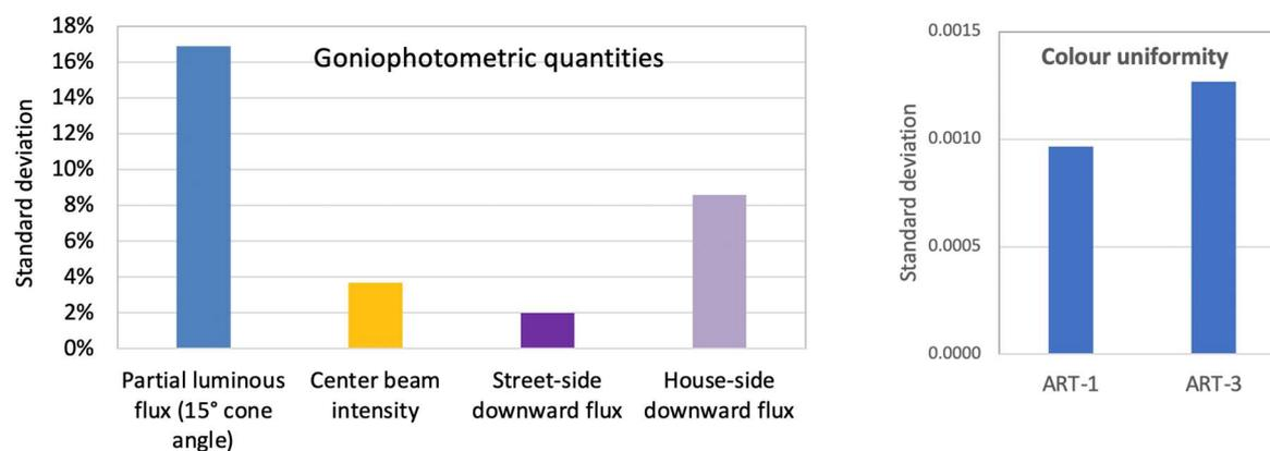
**Figure 7-67 Standard deviations of four goniophotometric quantities and colour uniformity**
