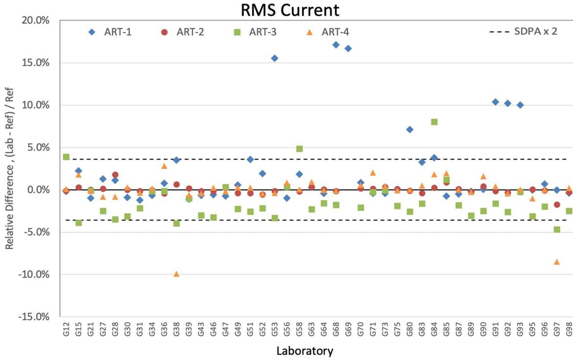
Figure 7-13. Relative differences of RMS current for all artefacts
