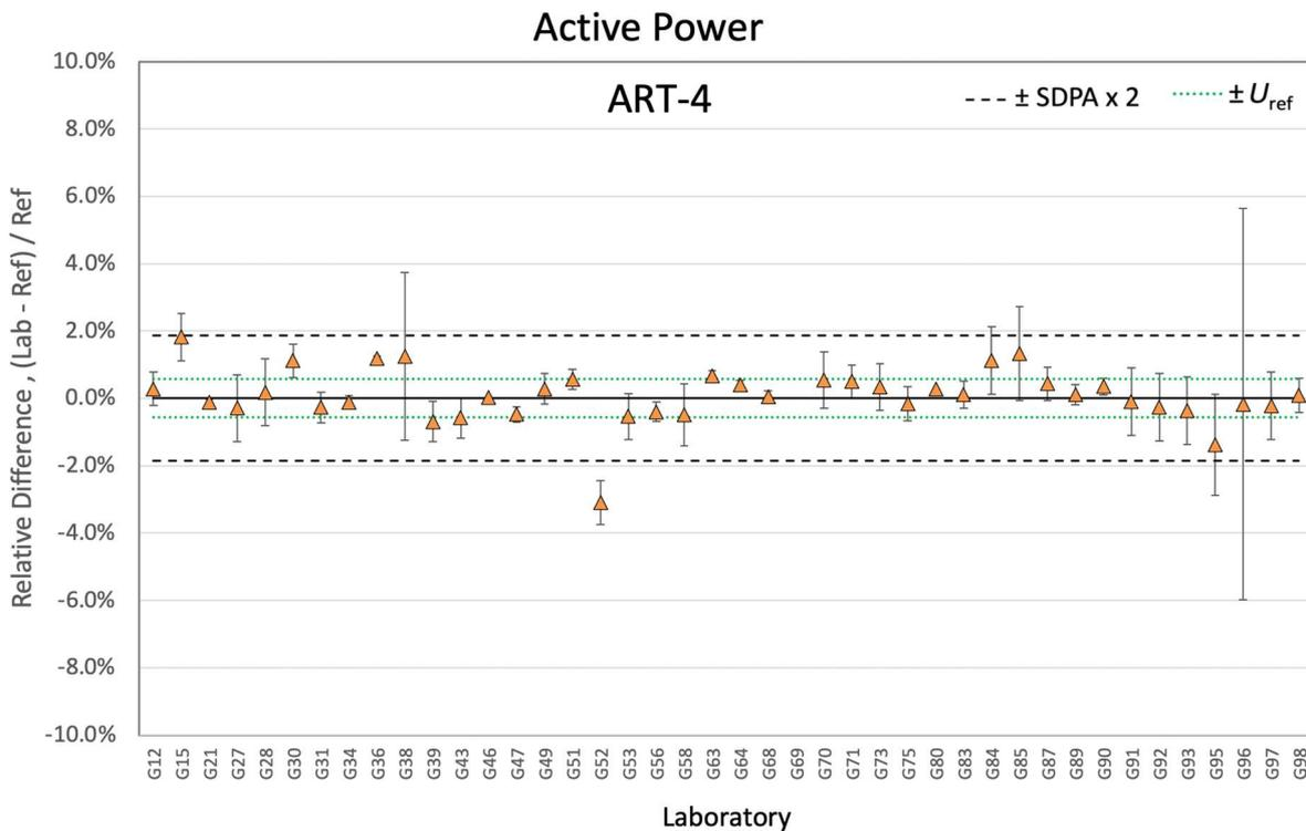
Figure 7-12. Relative differences of active power for ART-4
