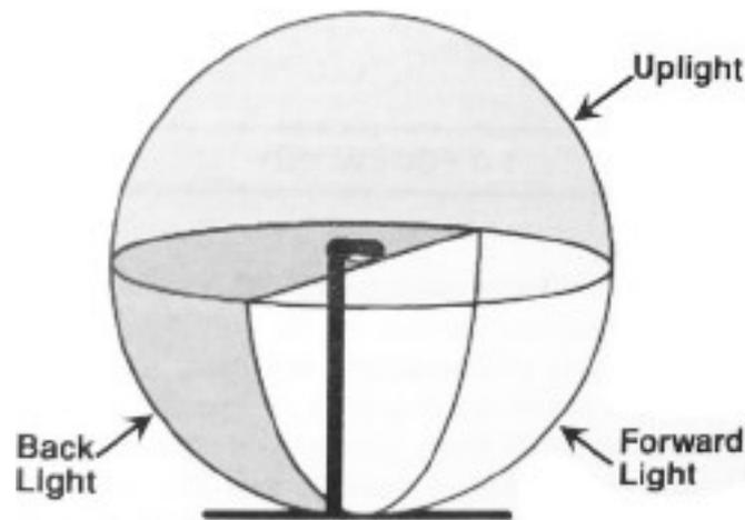
Figure 3-2. The three primary solid angles of the Luminaire Classification System (LCS) defined in IES TM-15
