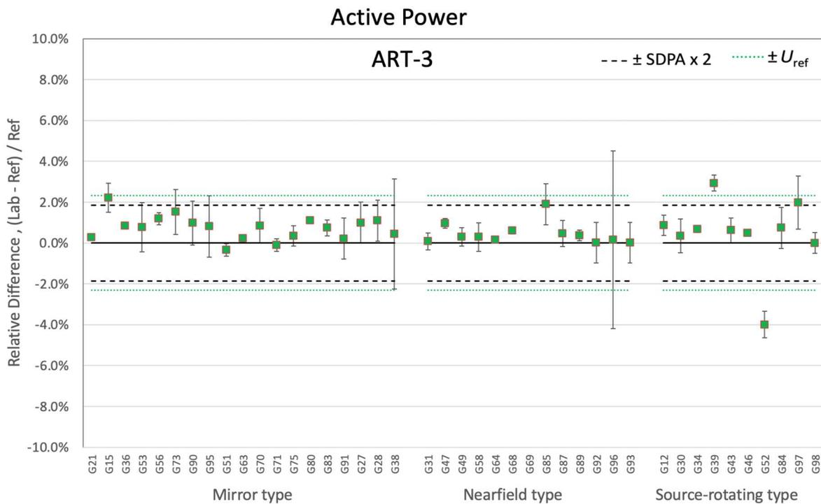
Figure 7-78. Relative differences of active power for ART-3 by goniophotometer type
