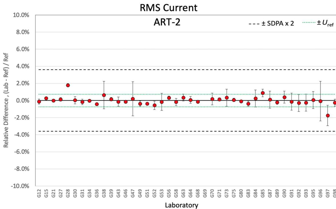
Figure 7-16. Relative differences of RMS current for ART-2
