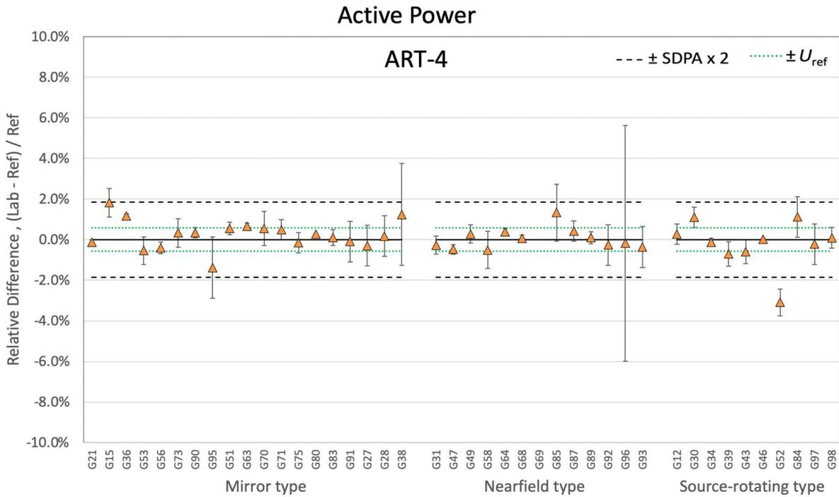
**Figure 7-79. Relative differences of active power for ART-4 by goniophotometer type**
