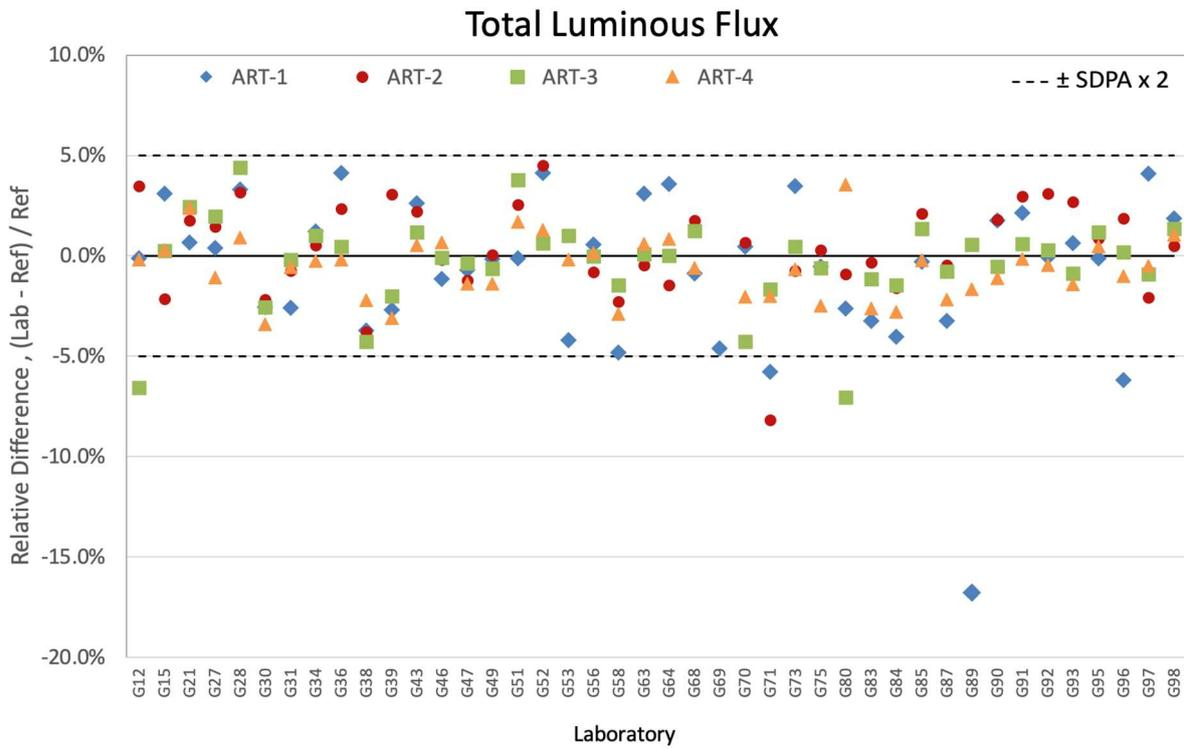
Figure 7-1. Relative differences of total luminous flux for all artefacts
