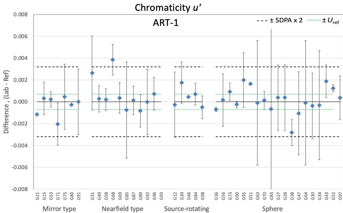
Figure 7-95. Differences of chromaticity  $u'$  for ART-1 by goniophotometer type and sphere
