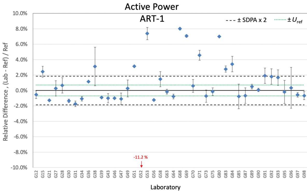
Figure 7-9. Relative differences of active power for ART-1
