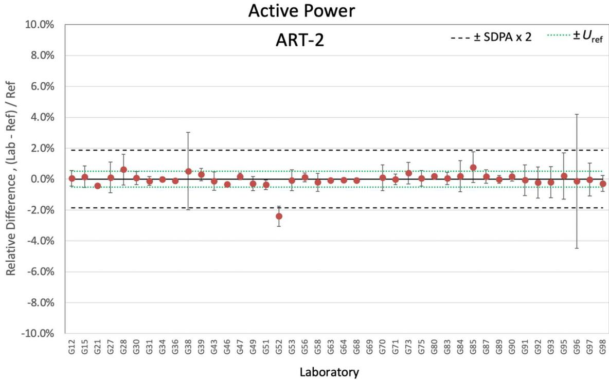
**Figure 7-10. Relative differences of active power for ART-2**
