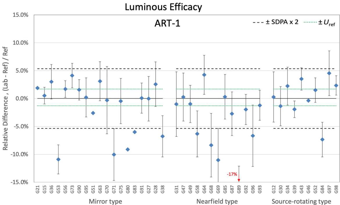
Figure 7-86. Relative differences of luminous efficacy for ART-1 by goniophotometer type
