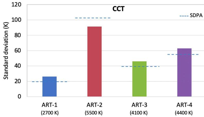
Figure 7-42. Standard deviations of CCT results
