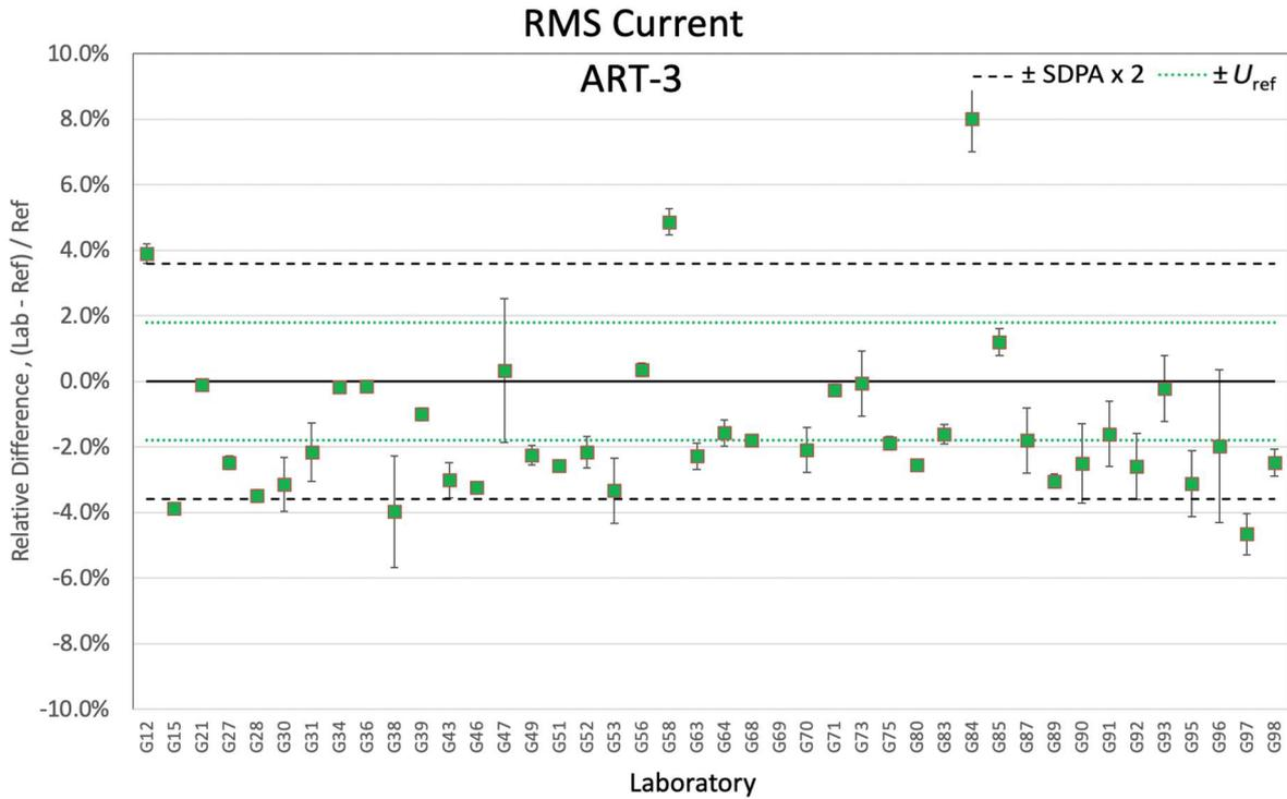
Figure 7-17. Relative differences of RMS current for ART-3
