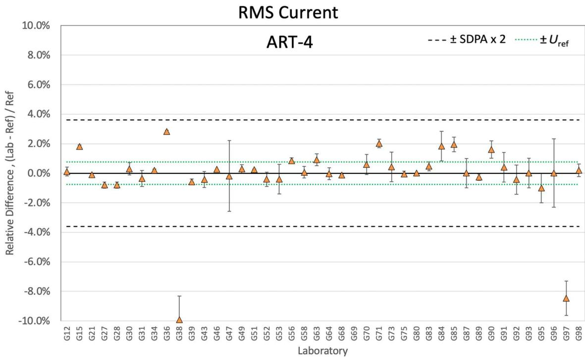
Figure 7-18. Relative differences of RMS current for ART-4
