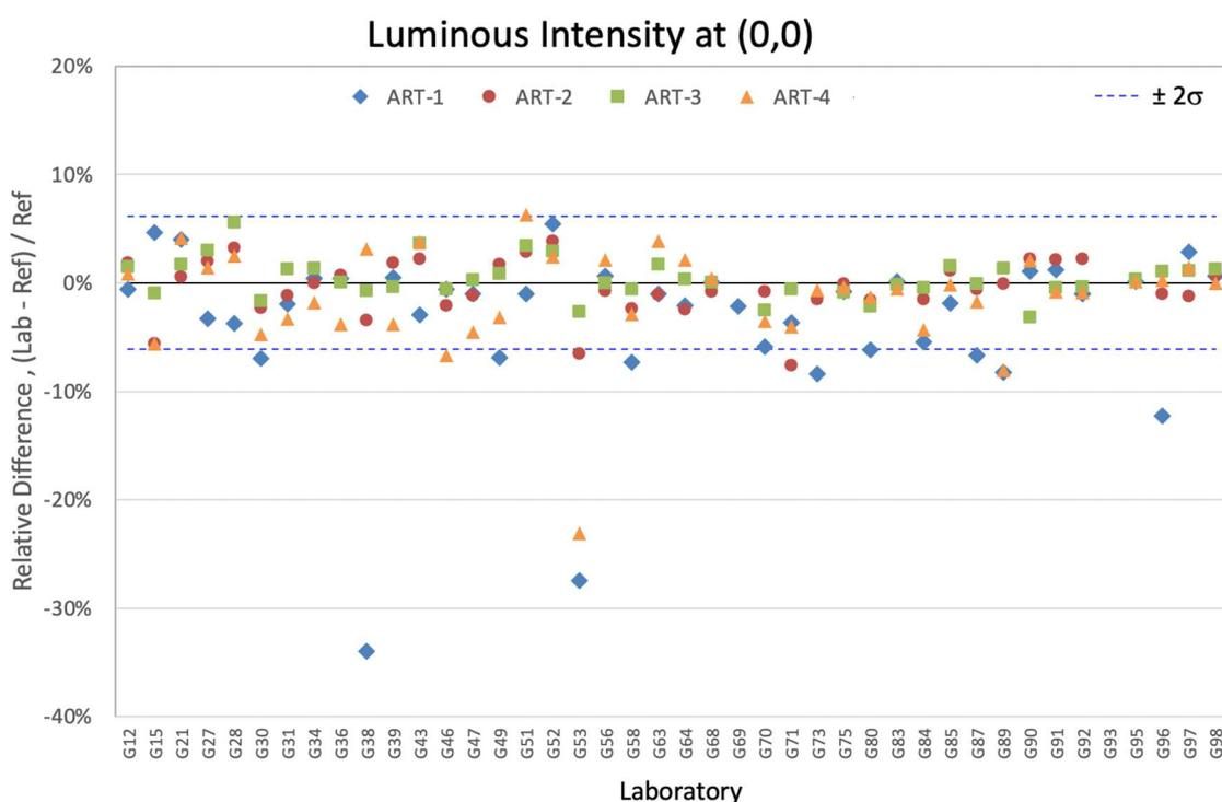
Figure 7-53. Relative differences of luminous intensity at (0,0) for all artefacts
