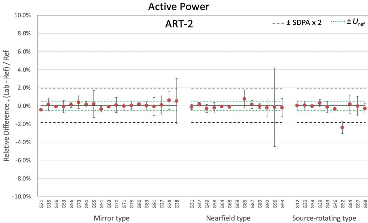
Figure 7-77. Relative differences of active power for ART-2 by goniophotometer type
