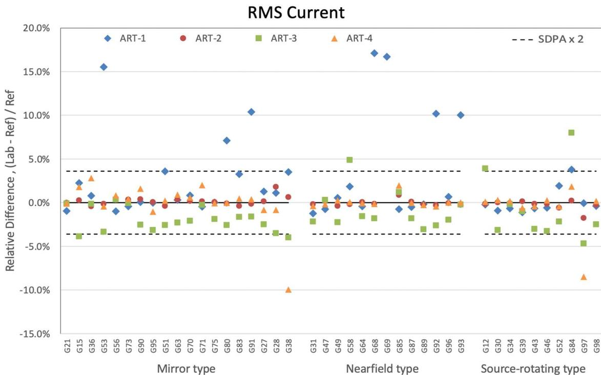
**Figure 7-80. Relative differences of RMS current for all artefacts by goniophotometer type**
