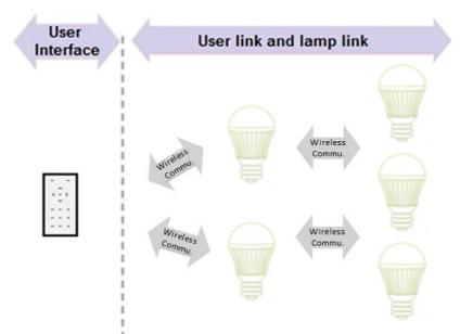
Figure 7. Communications architecture Type D using a remote control and a proprietary protocol
