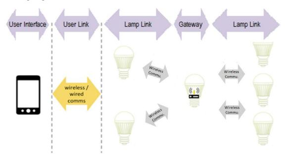
Figure 6. Communications architecture Type C using WiFi and one lamp including gateway that communicate to the other lamps using another protocol
