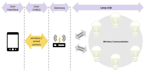
Figure 4. Communications architecture Type A using WiFi, gateway and another protocol
