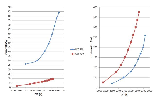
Figure 21. Comparison of DimTone LED lamp and 40 W incandescent lamp
