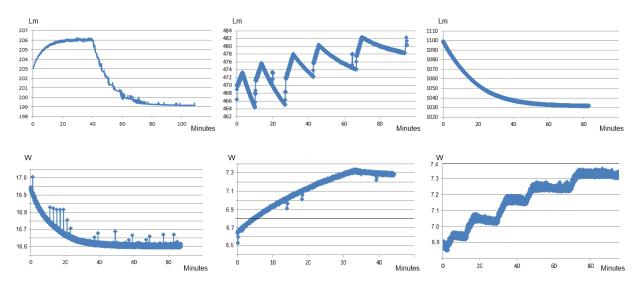
Figure 8. Examples of stabilisation measurements for luminous flux and power
