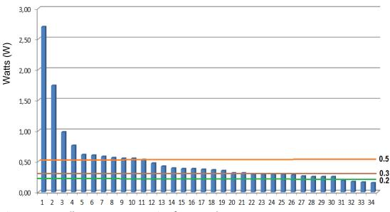
Figure 11. Standby power consumption for smart lamps
