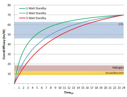
Figure 2. Example of variation in overall efficacy of three 10 W smart lamps providing 700 lm with different standby powers (1, 2 or 3 W) for all hours of ON usage per day
