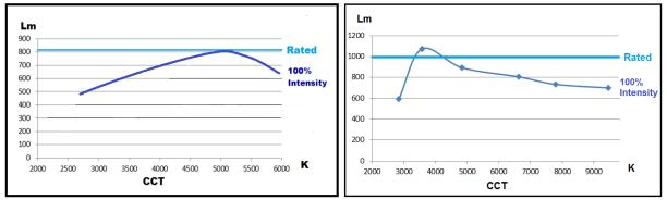
Figure 10. Two examples of measured total luminous flux as a function of CCT
