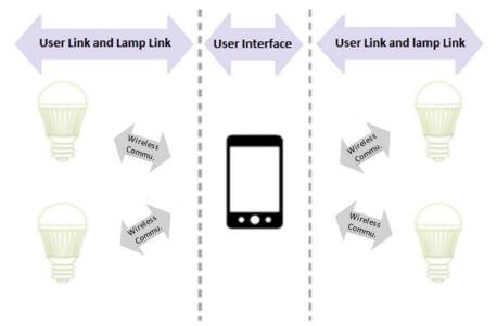
Figure 5. Communications architecture Type B based on either WiFi or Bluetooth
