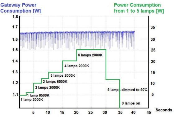
Figure 9. Nearly constant gateway consumption with a varying number of lamps in operation
